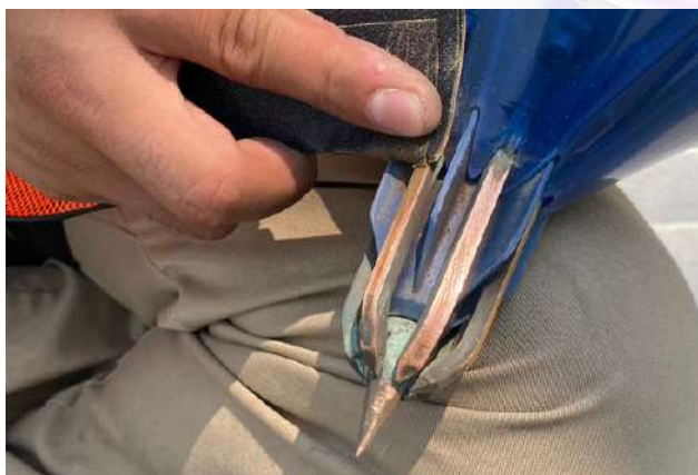
Head lightning protection cleaning
